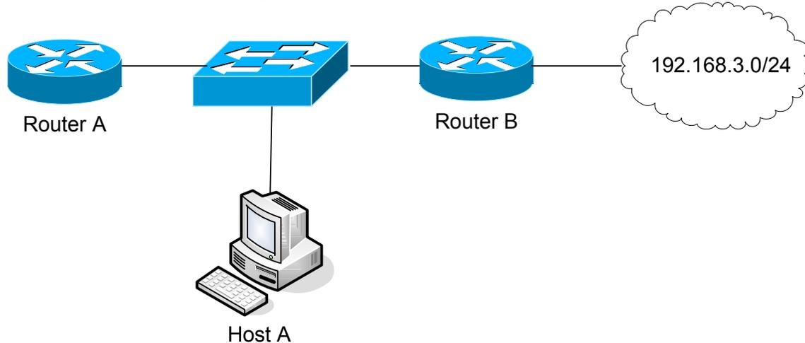
Consider the above example, and assume that the Host points to Router A as its default gateway. When the Host sends a packet destined to 192.168.3.0, it will forward it first to Router A, which then forwards it *out the same interface again* to Router B.
