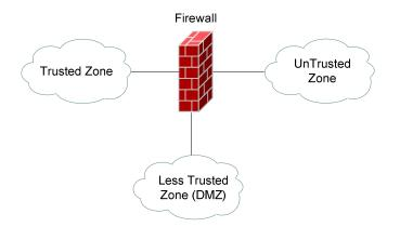
To control the *trust* value of each zone, each firewall interface is assigned a *security level*, which is often represented as a numerical value or even color. For example, in the above diagram, the Trusted Zone could be assigned a security value of 100, the Less Trusted Zone a value of 75, and the Untrusted Zone a value of 0.
