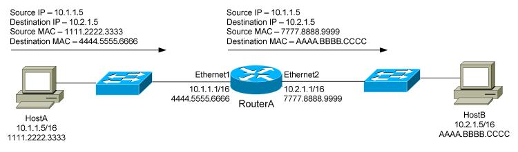
Note that as a packet is *routed*, the source and destination IP address remain unchanged. However, both the source and destination MAC address *did* change.
