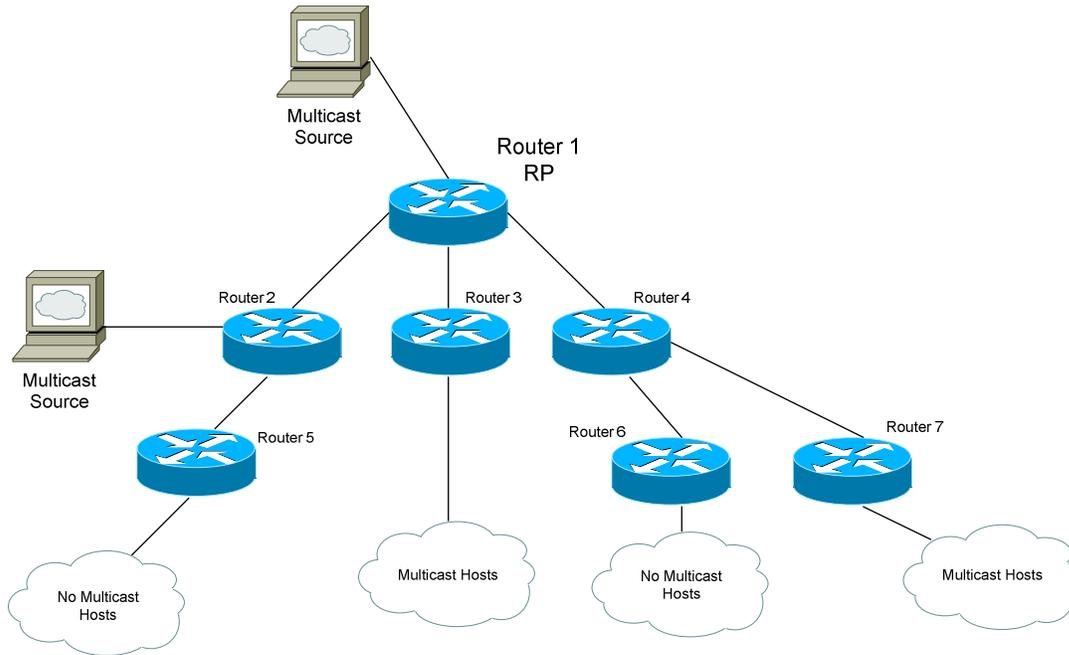
When PIM routers operate in **Sparse Mode**, multicast traffic is *not* initially flooded throughout the entire multicast tree. Instead, a Rendezvous Point (RP) is elected or designated, and all multicast sources and clients must explicitly register with the RP. This provides a centralized method of directing the multicast traffic of multiple multicast sources:
