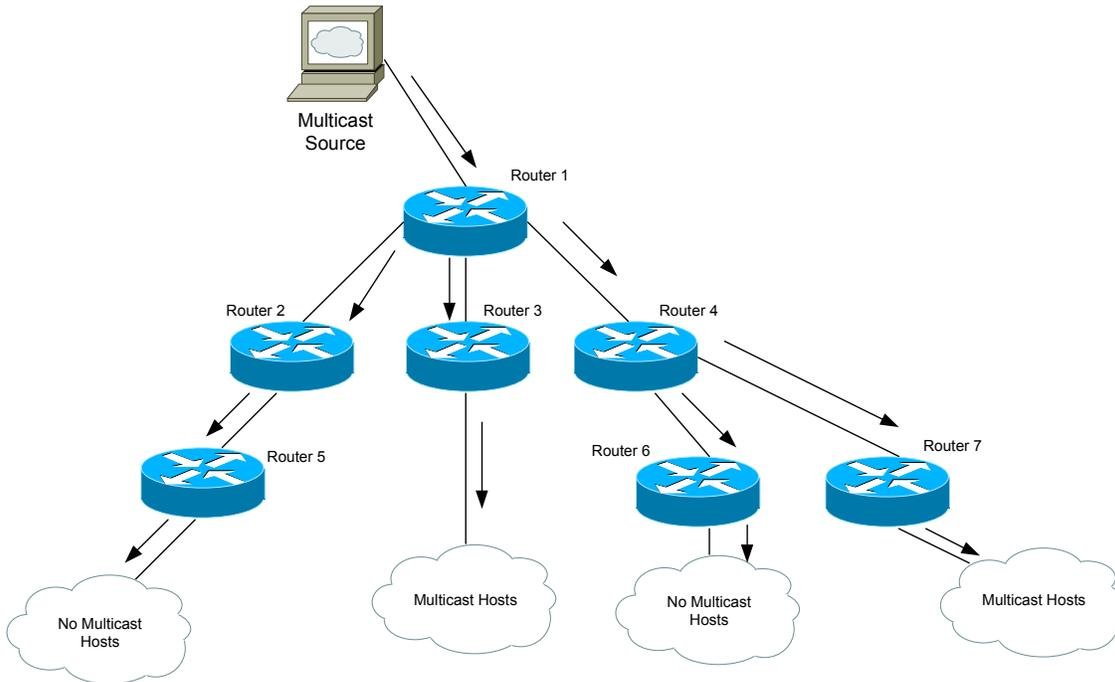
Consider the above example. When PIM routers operate in **Dense Mode**, all segments of the multicast tree are flooded initially. Eventually, “branches” that do not require the multicast traffic are pruned off:
