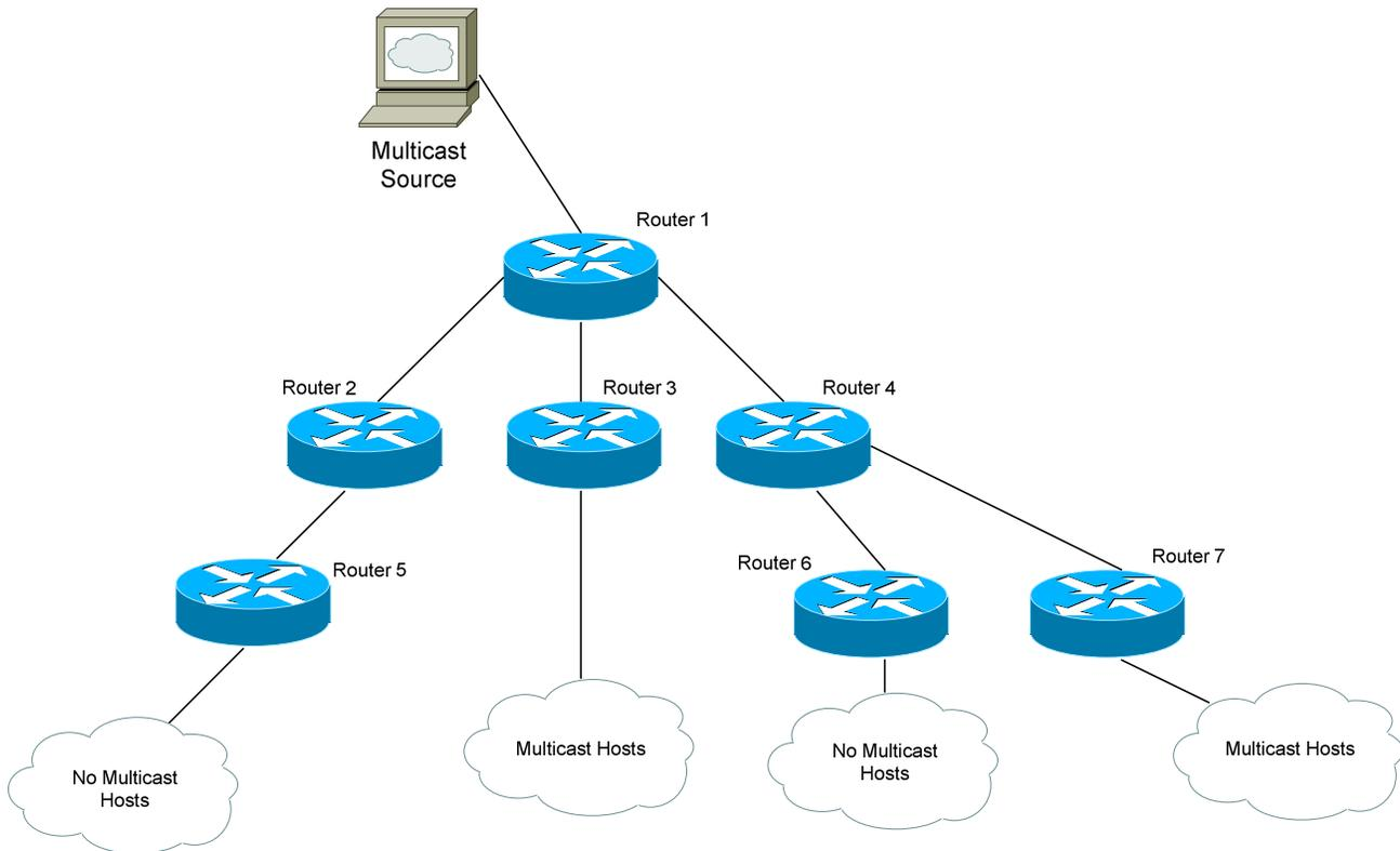
A router interface will not be designated as a **downstream** interface unless multicast hosts actually exist downstream. In the above example, no multicast hosts exist downstream of Router 5.
