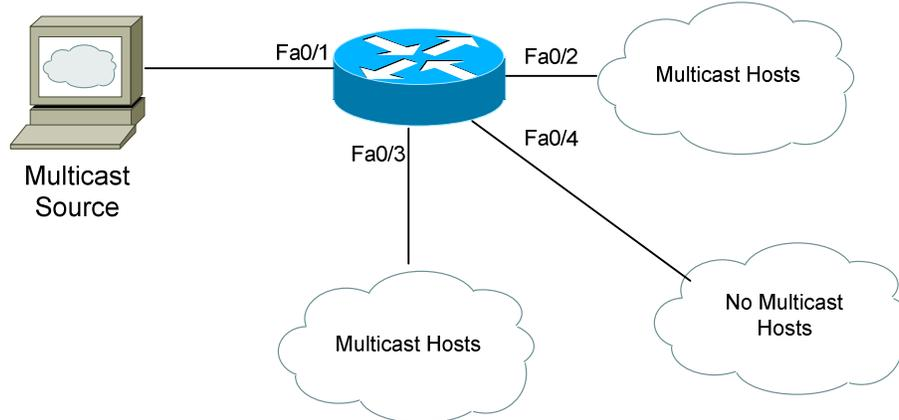
In the above example, assume the router is using IGMPv2. Interface fa0/1 points towards the multicast source, and thus becomes the **upstream** interface.
