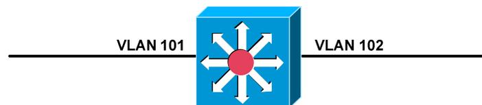
**Multilayer switching** is a generic term, encompassing any switch that can forward traffic at layers higher than Layer-2.
