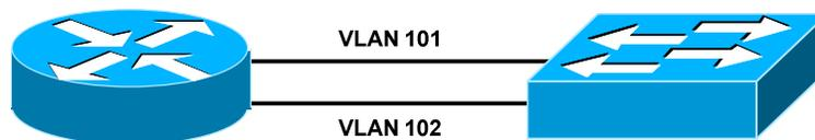
The second method involves using an **external router** with a single **trunk link** to the switch, over which all VLANs can be routed. The router must support either 802.1Q or ISL encapsulation. This method is known as **router-on-a-stick**:
