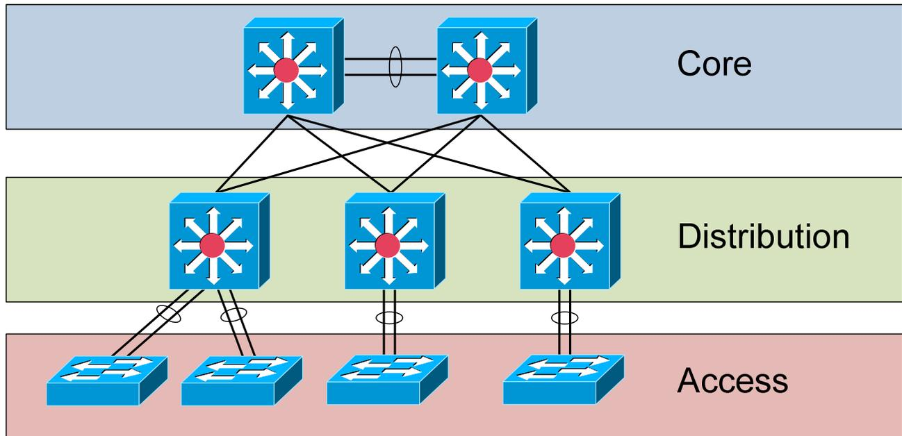
The **access layer** is where users and hosts connect into the network. Switches at the access layer typically have the following characteristics:
