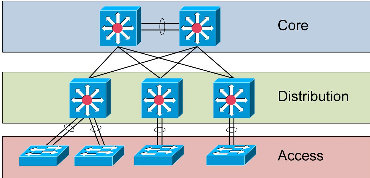
The **core** layer is responsible for connecting all distribution layer switches. The core is often referred to as the **network backbone**, as it forwards traffic from to every end of the network.
