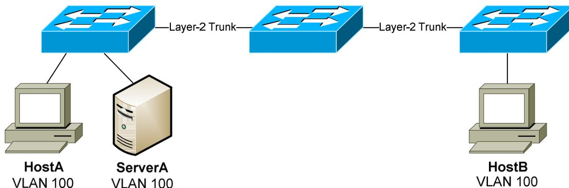
End-to-end VLANs allow a host to exist *anywhere* on the campus network, while maintaining Layer-2 connectivity to its resources.
